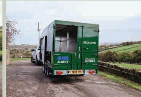
As a fresh pair of eyes in the industry, we saw an area in which could be improved drastically, which is the need for multiple unit trailers for different unit base requirements on set. In reaction to this, we created our own unit trailer containing a rubbish trailer divided into recycling and general waste at the back, and fresh water bowser and waste water bowser at the front, all within one unit trailer. This allows us to offer a much more eco-friendly option to productions.
